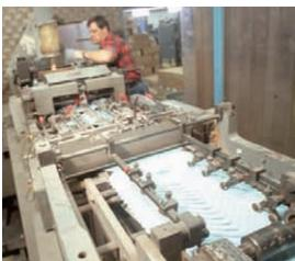
(Left) Furniture manufacturers use vacuum in place of traditional clamping methods to avoid damage.
