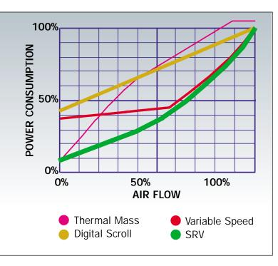
The chart above compares three of the most energy efficient dryers to the Sullair SRV. No other single method of drying compressed air is able to provide the operational efficiencies across the full range of air flow as does the SRV.
